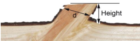
Figure 6. Measurement of height of branch stub and fork.
